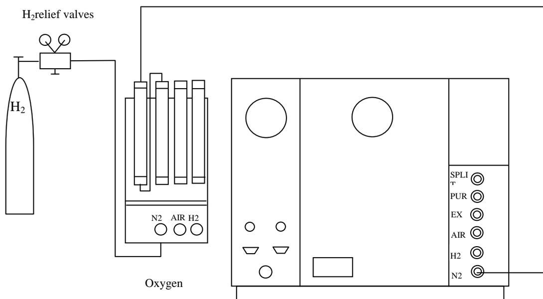
7-8 GC1120-TCD Connection Diagram of outer Gas Path
