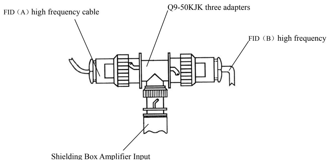
Figure 3-6 Connection Diagram Of Double FID Compensation High Frequency Cable
