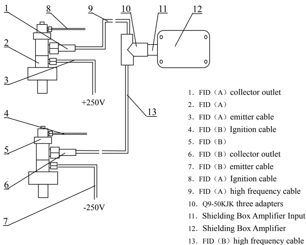
Figure 3-5 Double Connection Diagram Of Double Detector
