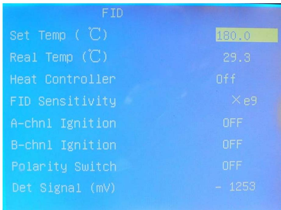
Use PgUp or PgDn to select the item. Then press [EDIT] to change to edit mode. Use number key to input data and [ENT] to finish setting.
