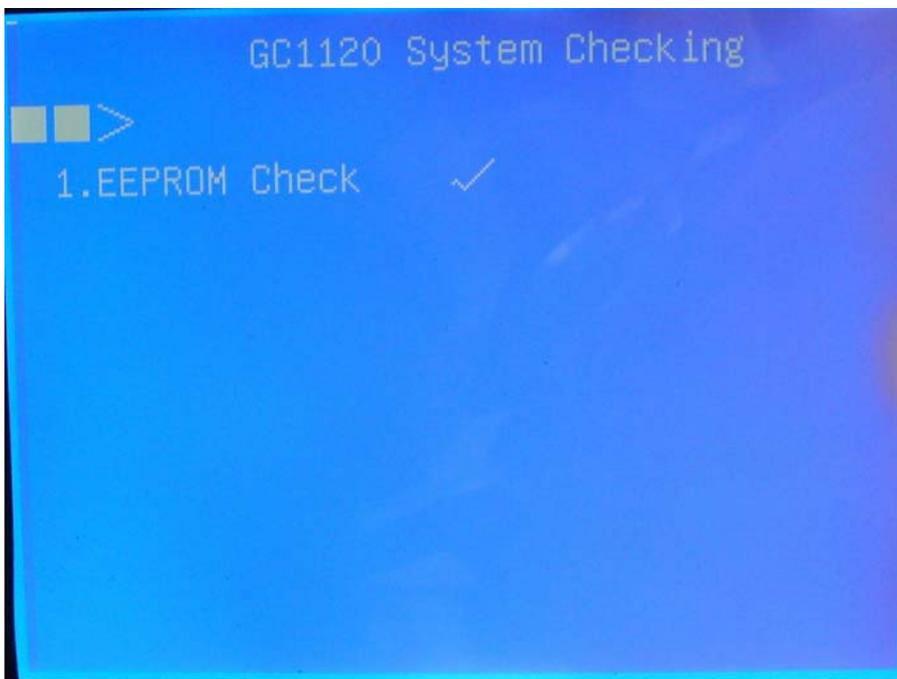
4 items will be checked as shown in figure below. And the 3<sup>rd</sup> is for back door of oven. Error for this item is not a problem, it only means the back door open when power on. And it will be closed automate.
