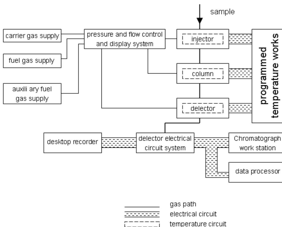
Figure 1-1 GC1120 Gas Chromatograph Working Scheme
