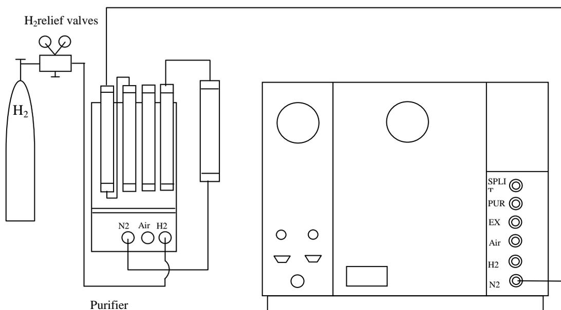
Figure 7-9 De-oxidation tube connection sketch
