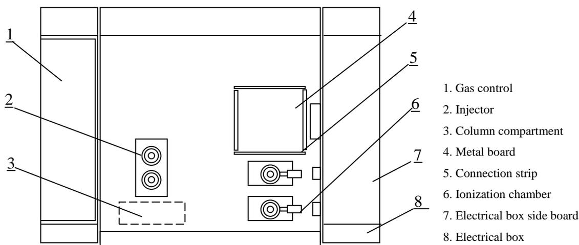
Figure 7-3 Mainframe top view
