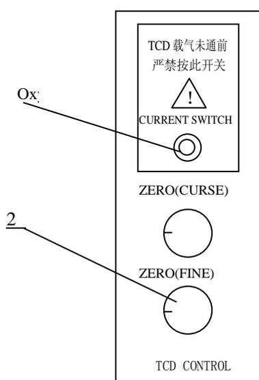
Figure 7-7 GC1120-TCD current regulator panel layout
