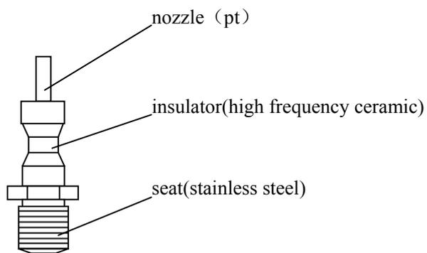
Figure 3-2 Nozzle Structure
