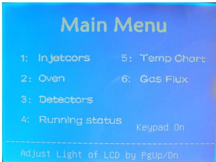
In main menu, number keys 1-7 used to select items. PgUp and PgDn keys set the light of the screen. When [LOCK] key pressed, “Keypad On” at the right corner of the screen will change to “Keypad Off”
