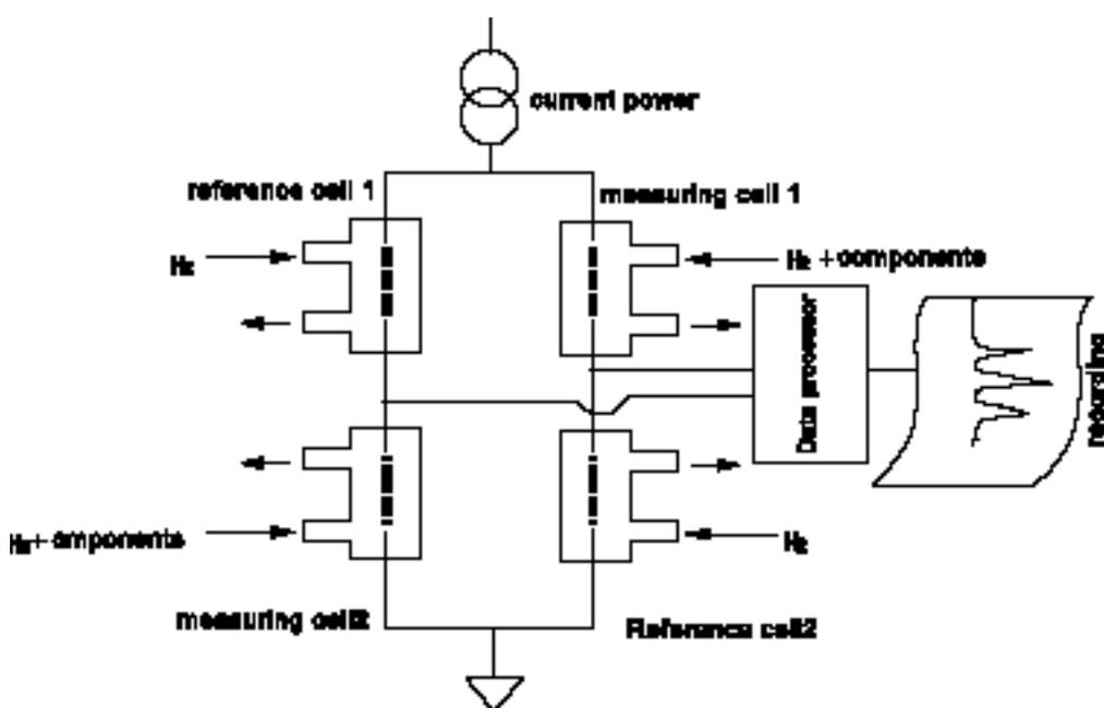
Figure 7-2 GC1120-TCD working principle sketch
