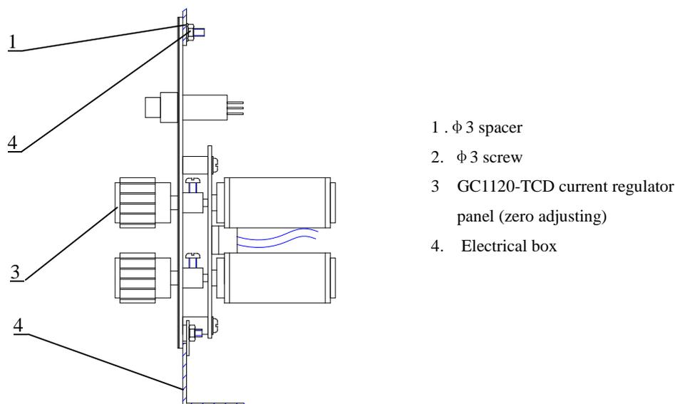
Figure 7-5 Schematic drawing for parts under the electrical box
