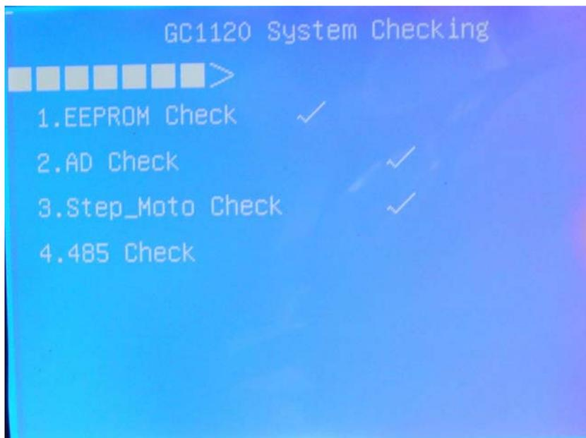
After self-check finished and no error, two beeps can hear and screen will go into main meun.
