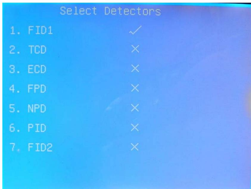
All detectors GC1120 can be installed will display on this screen. And a ✓ mark display on the item if the detector was installed. Detectors installed can be automatic checked when power on.
