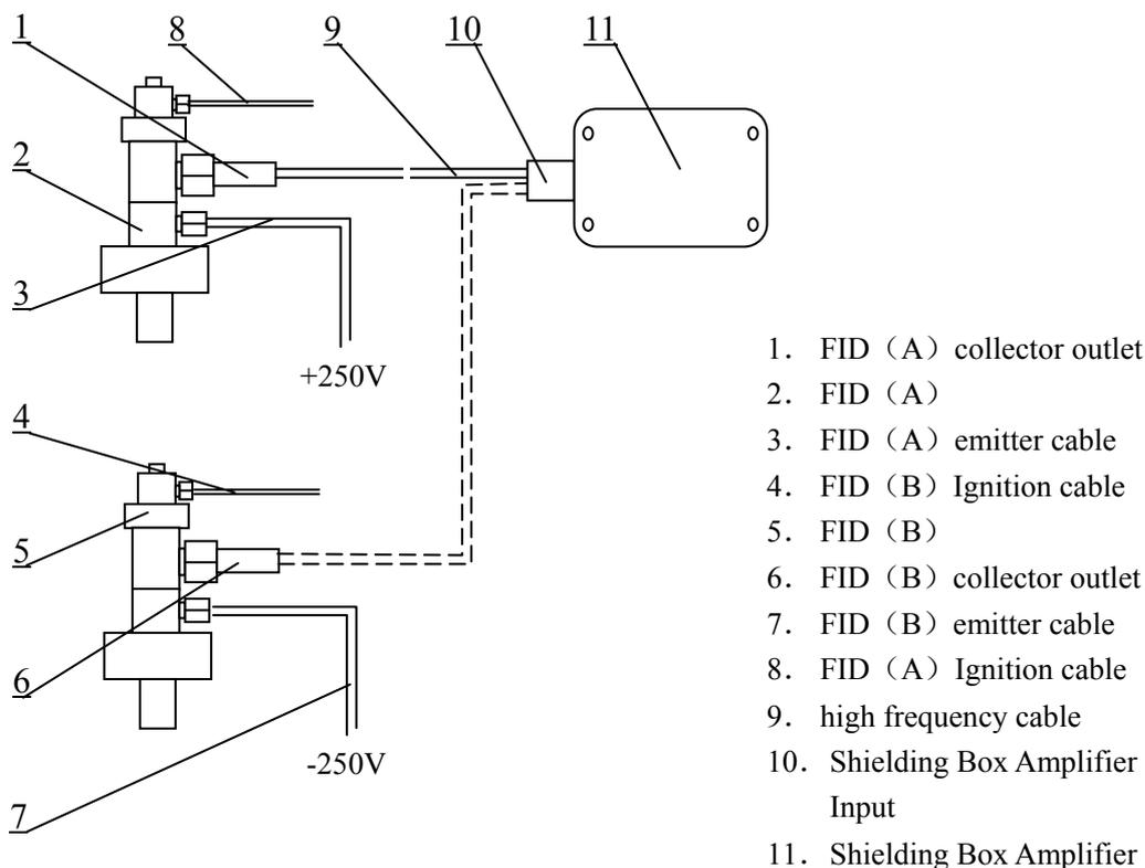
Figure 3-4 Signal Connection Diagram Of Single Detector
