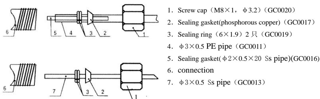
Figure 4-2 Connection Diagram Of Outer Gas Path Joint
