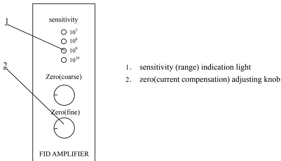
Figure 3-7 FID micro current control amplifier panel diagram
