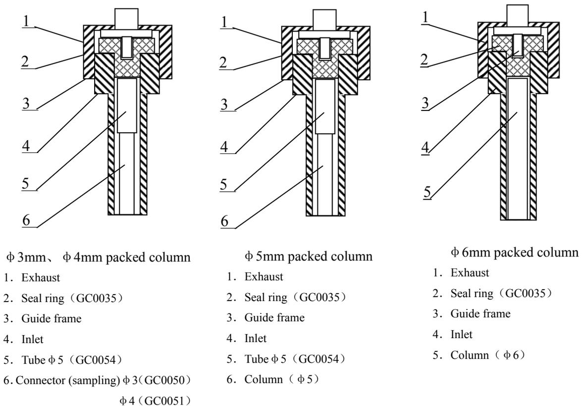
Figure 1-4 Packed column inlet (part)
