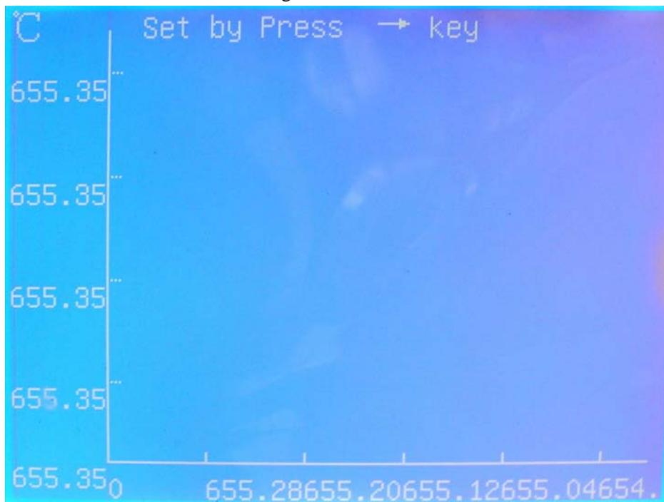
On this screen, temperature curve will display. This is useful for program temperature. Use right arrow key into curve display parameters setting screen. On setting screen, max and min temperature displayed and sampling frequency can be set. Use PgUp or PgDn to select the item. Then press [EDIT] to change to edit mode. Use number key to input data and [ENT] to finish setting.
