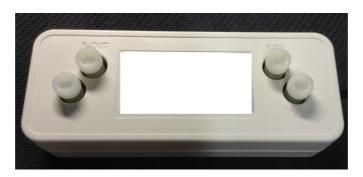
E-IN: Eluent inputR-IN: Regenerated solvent inputR-OUT: Eluent outputR-OUT: Regenerated solvent output
