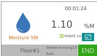
▷ When select timing mode, moisture analyzer will stop the measurement and revert back to complete moisture measuring interface when reach to pre-setting time.
