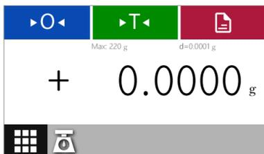
► Switch to other weighing unit, please click unit button (like “g”) on weighing interface.
