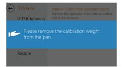
► Remove the calibration weight from the weighing pan according to the hints, empty pan.
