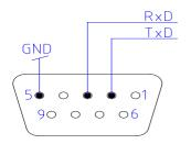
Every balance could connect peripheral equipments with RS-232C interface (like nine-pin serial printer and micro-computer). Once connect with printer, could press to output weighing result according to the print settings.
