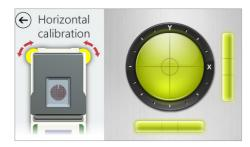
Through adjusting levering feet behind, to place the levering bubble in the right Center (refer to Page 28 for detail processing)
